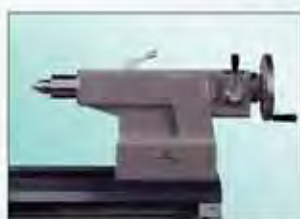
▲ Tailstock hand-wheel has two-speed feed
